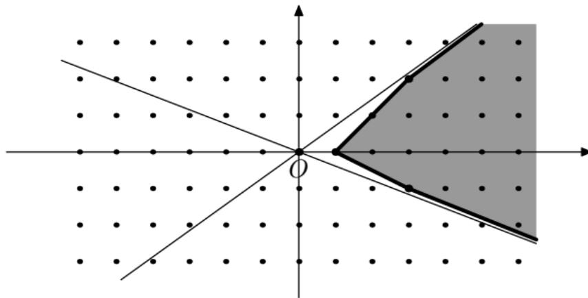
The *sail* for one of the octants, i.e. the boundary of the convex hull of all integer inner points.
